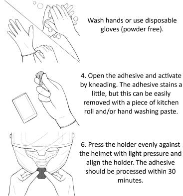
6. Press the holder evenly against the helmet with light pressure and align the holder. The adhesive should be processed within 30
